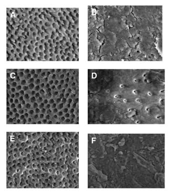
**Figure 1.** Scanning electron micrographs of the middle aspect of root canals. (*A*) F-file: 6% NaOCl and 17% EDTA, (*B*) F-file: 6% NaOCl, (*C*) ultrasonics: 6% NaOCl and 17% EDTA, (*D*) ultrasonics: 6% NaOCl, (*E*) 6% NaOCl and 17% EDTA, and (*F*) saline.
